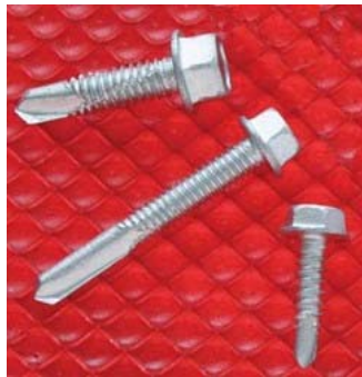
Bi-Flex 300 Series SS Fasteners: 12-14 x 2", 5/16" Hex Head, #2 Point, Box of 200
