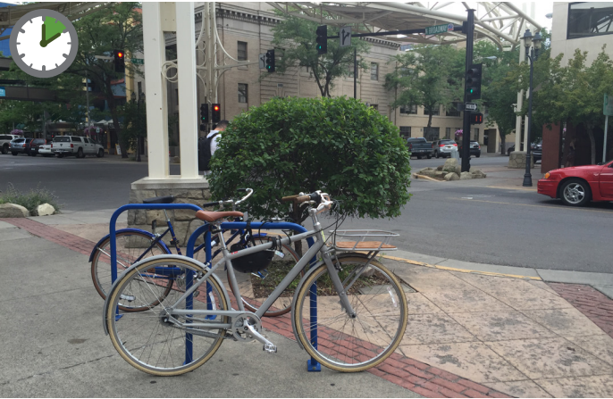
Tier 1: Short-Term Bicycle Parking: Short-term bicycle parking is to be placed on sidewalks in front of higher turn-over establishments, or near the entrance to buildings on private property.
