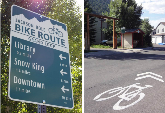
Jackson Hole, WY, bicycle boulevard network has been implemented economically, using signage and pavement markings.
