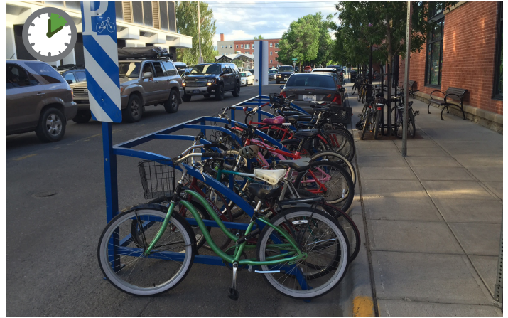
Tier 2A: Bicycle Corral: On-street bicycle corrals provide high-capacity parking outside of the pedestrian zone, helping to minimize sidewalk clutter. This rack type should be installed at locations with high demand, such as near downtown entertainment areas.
